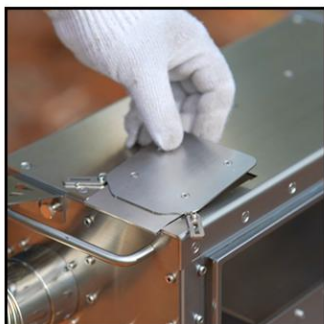
Install the cover plate
