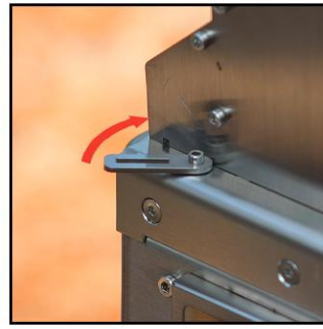
Push in the buckles on both sides to fasten the pellet tube
